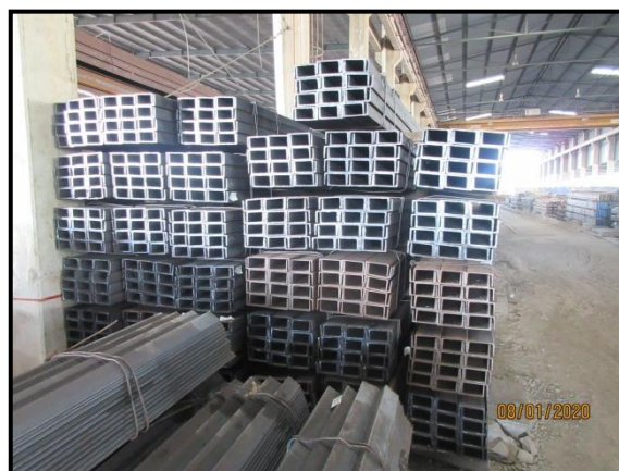
HOT ROLLED SECTIONS OF NON –ALLOY STRUCTURAL STEEL (150 X 75 X 6.5)MM X 6M
